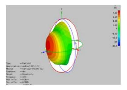
Figure 4(b): 3-D Radiation Pattern at 3.45 GHz
