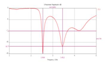
Figure 2: Return Loss verses Frequency Graph
